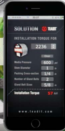
iPhone app for installation torque
